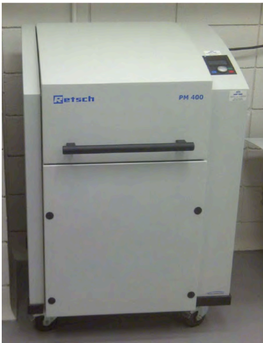
Retsch centrifugal ball mill (agate jars and balls)
