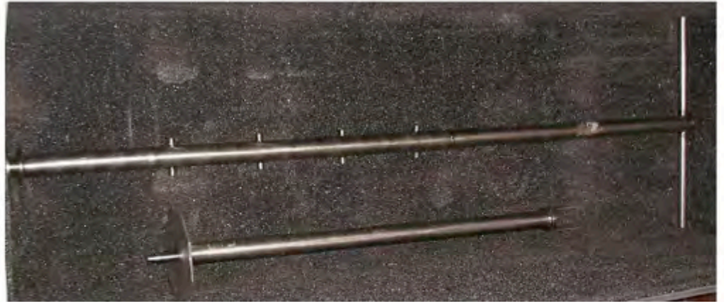
Modified Wardeaar peat monolith corer, titanium
