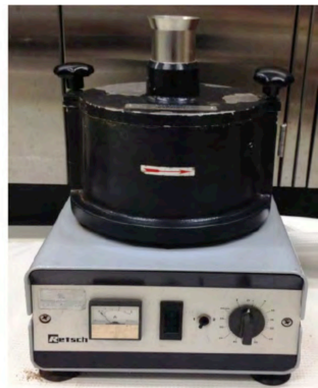
Retsch titanium ultracentrifugal mill
